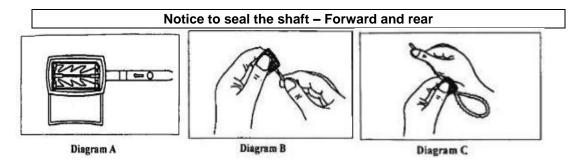
Step 1 Make sure the seal flap is placed with the front side facing the user as shown in diagram A
